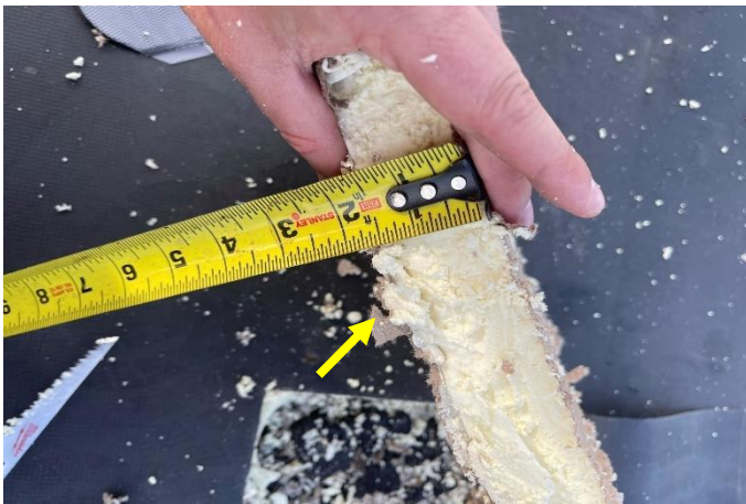
View of core-cut taken on Roof Area C. The single-ply roofing system consists of a mechanically attached EPDM membrane with 1.50" of polyisocyanurate. No moisture was documented at core-cut location. Picture #5
