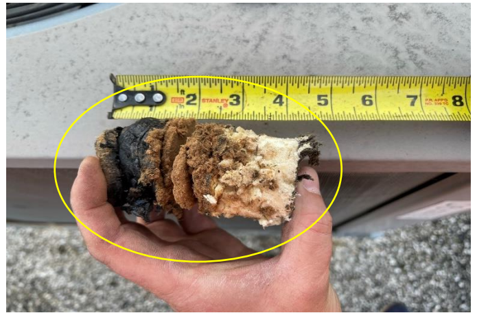
View of core-cut taken on Roof Area C. The roof consists of a mechanically attached EPDM roof, 1.50" polyisocyanurate insulation, gravel asphalt built-up roof, 1.00" wood fiber board, 1.50" polyisocyanurate insulation and a steel deck. Picture #6
