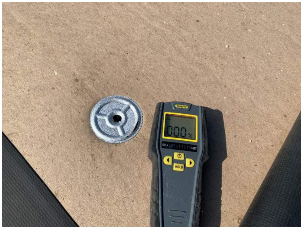
Photo #26 – No moisture reading at Invasive Location #4
