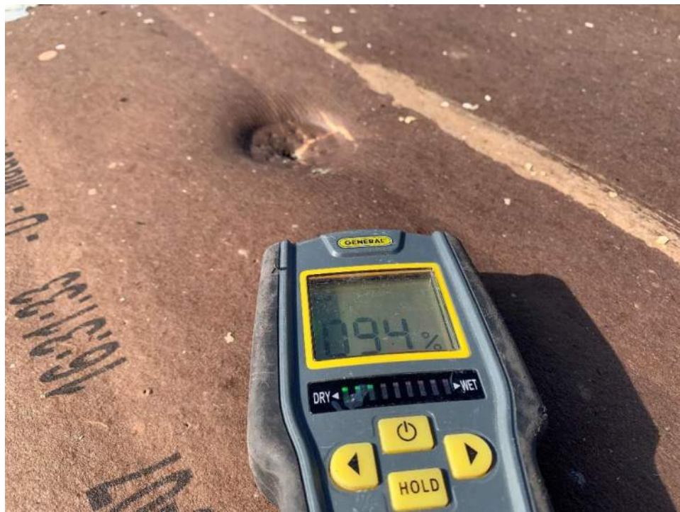
Photo #16 – Moisture reading below top layer of roofing at Invasive Location #1
