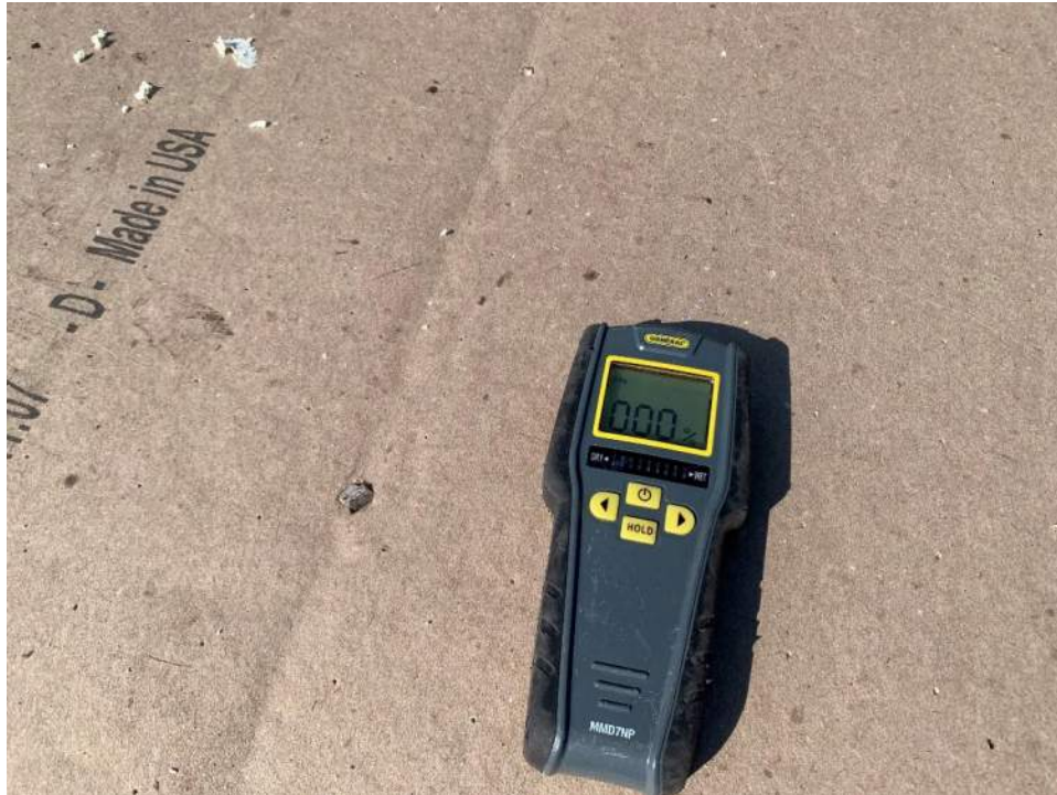
Photo #23 – No moisture reading at Invasive Location #3
