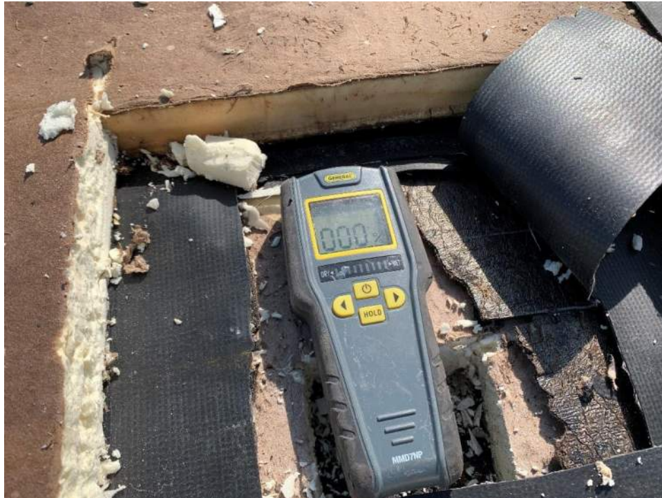
Photo #17 – No moisture detected below middle layer of newly installed roofing at Invasive Location #1
